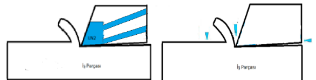
Figure 4. Internal cooling of the tool in the orthogonal cutting plane and cooling of the part and the cutting planes during cutting
