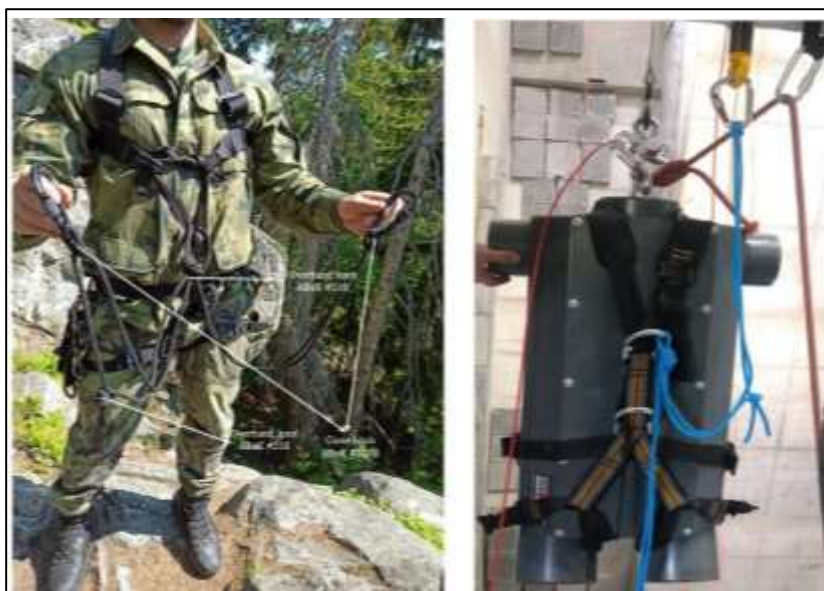
Picture 2. Improved via ferrata set made from 6mm reep cord and its lab variant
