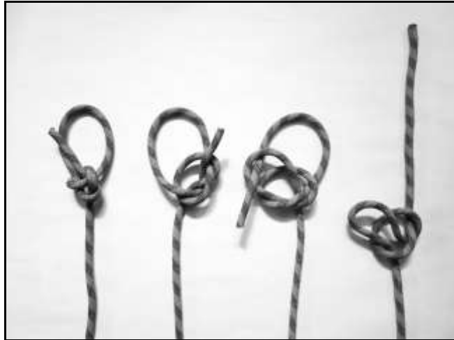
Figure 12. A Bowline without a backup knot capsizing, leaving a Running Overhand Slip Loop. The wend then Keeper migrates and releases forming an Overhand Slip Loop.
