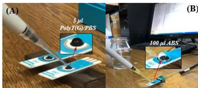
Figure 2. (A) Measurement anti-miRNA solution drop on the working electrode of SPE and (B) ABS solution drop on SPE during the measurement.
