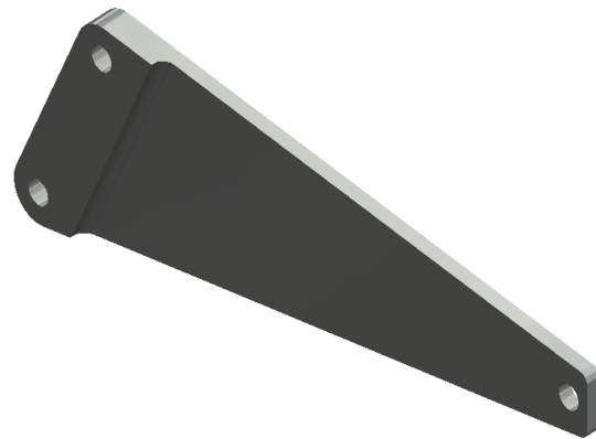
Figure 2. The solid model of the load-carrying element
