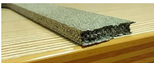
Figure 11. Specimen 1 (wall+lattice structure)
