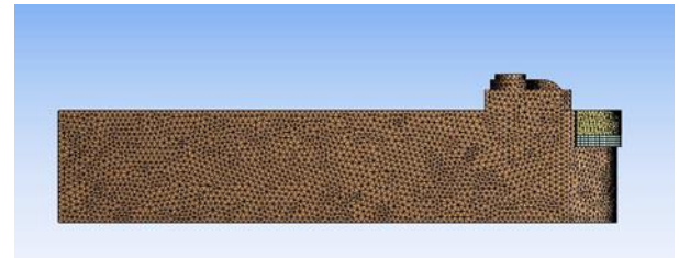
Figure 5. Elevation view of the grid generation.
