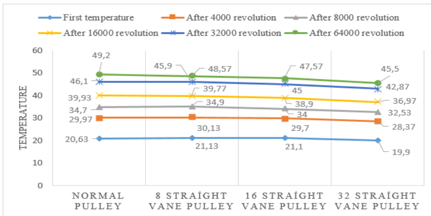
Figure 6. V-Belt temperature at straight vanes pulley
