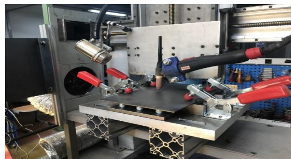
Figure 5. Infrared thermometer (IR) to measure temperature profiles
