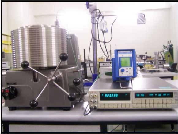
Fig. 3 Negative pressure drop system by pressure balance
