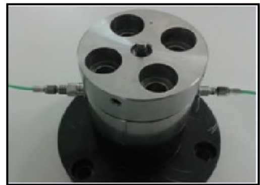
Fig. 13 Piston-cylinder with reference and test sensors
