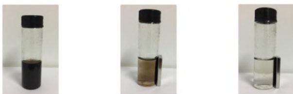
Fig. 2. Synthesized 0.5% w/v agar coated magnetic particles with an external magnetic field after (a) 0 s, (b) 15 s and (c) 71s
