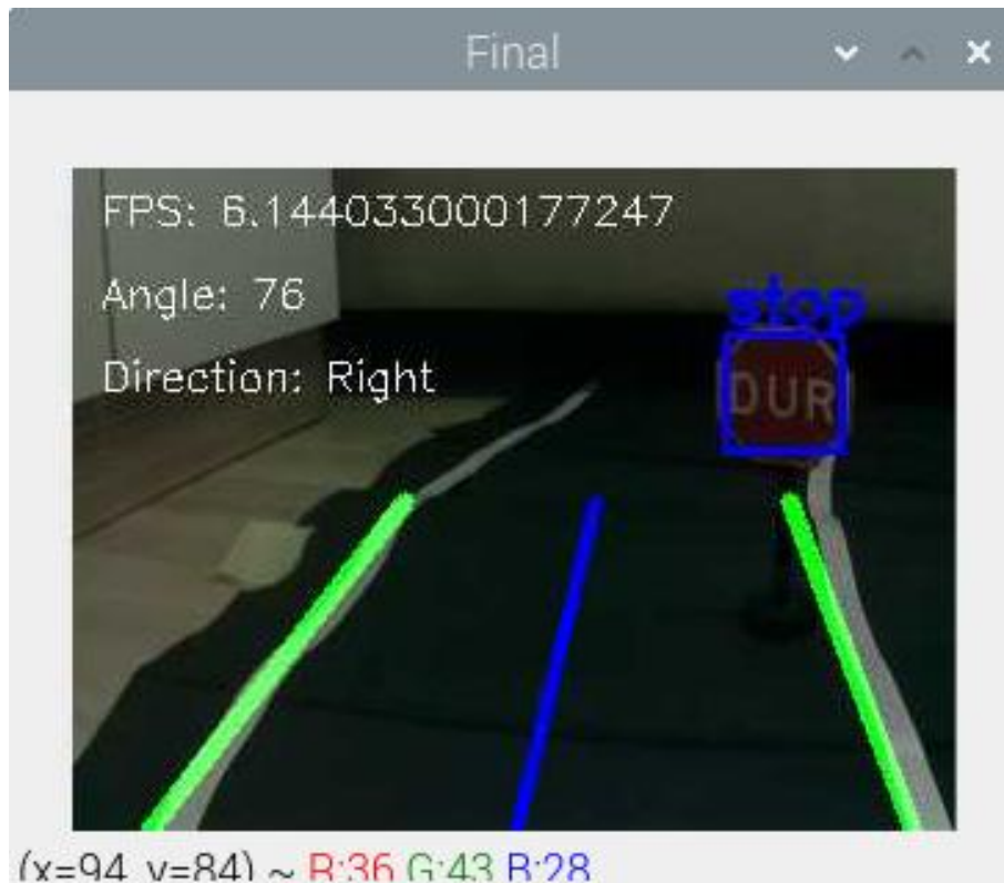
Figure 14. Recognition of 'Stop' traffic sign by using Haar Classifier with AV on the prepared dataset
