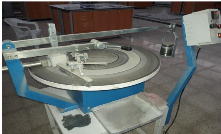
Figure 1. Böhme experimental setup
