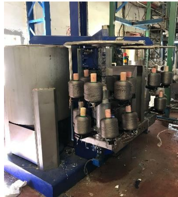
Figure 1. Yarn bobbin centrifugal dryer
