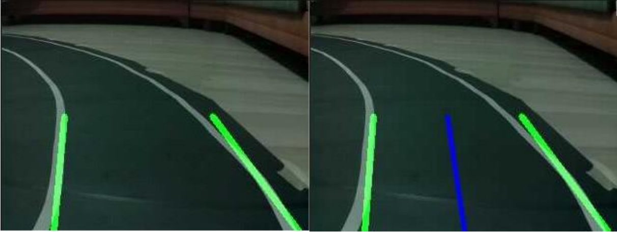
Figure 12. Determination of the tracking vector
