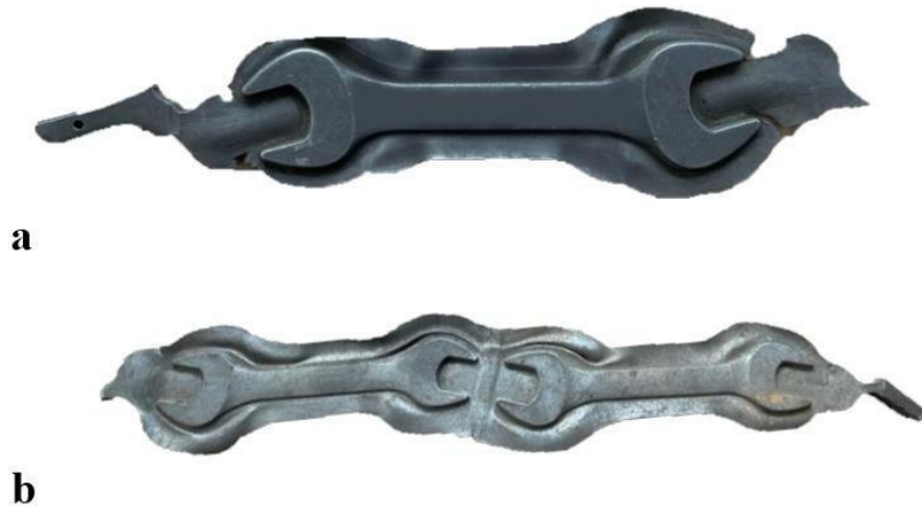
Figure 7. Single (a) Dual (b) 25 × 28 mm double-ended open-jaw wrench short pattern final shape after hot forging
