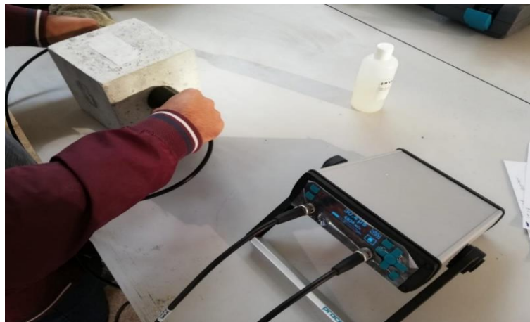
Figure 2. Ultrasonic transmission rate determination
