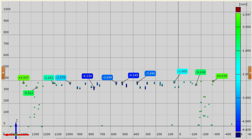
Figure 8. Displacement distribution under the 200 N load measured with GOM Tritop
