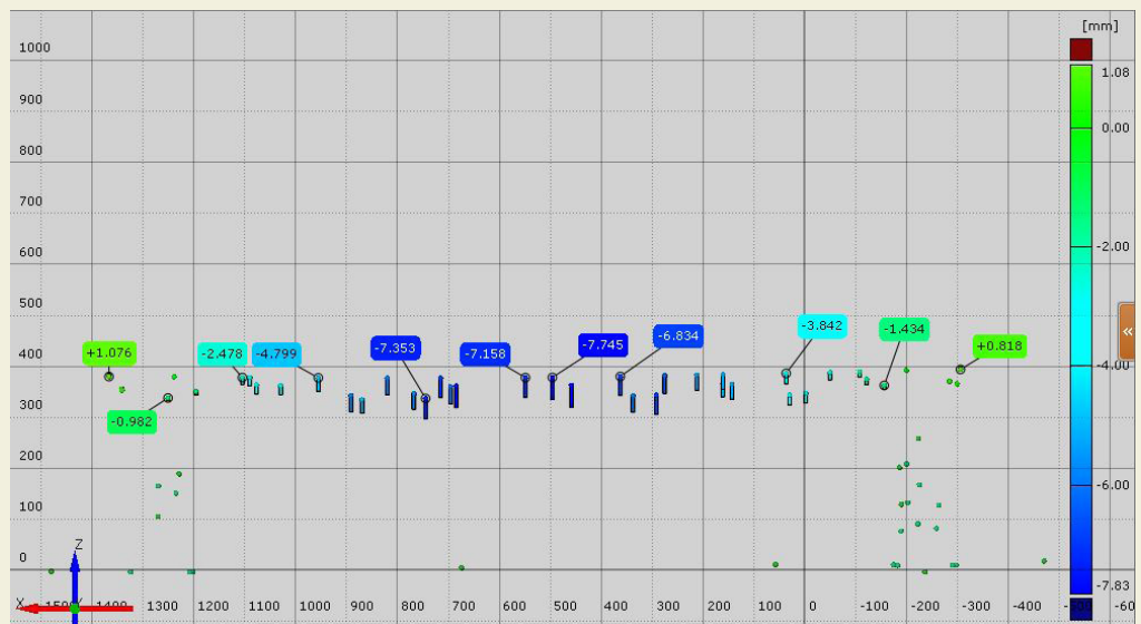
Figure 9. Displacement distribution under the 400 N load measured with GOM Tritop
