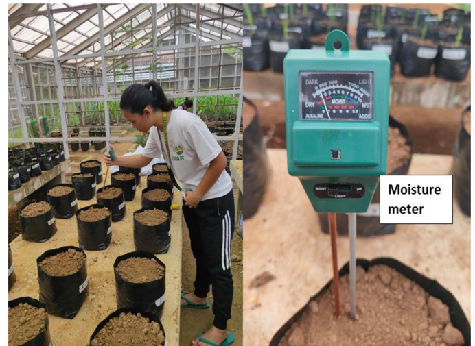
Figure 1. Preparation of the Pots for Nursery Experiment Using Clay Loam Soil with Less than 10%MC (dry soil/drought condition) as a Medium for Peanut Germination Study.
