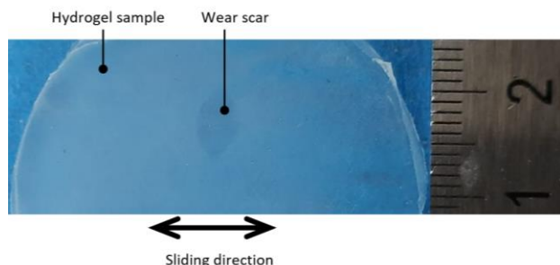
Figure 3. An illustration of wear track for 30%-DN hydrogel under 5 N.
