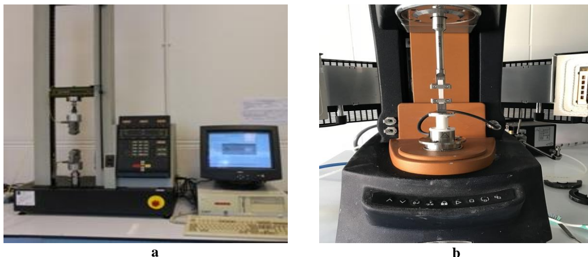
Figure 1. The devices used for tensile testing; a) the Instron 5564 Universal Testing Machine and b) the Hybrid Rheometer Discovery HR-2 Machine.
