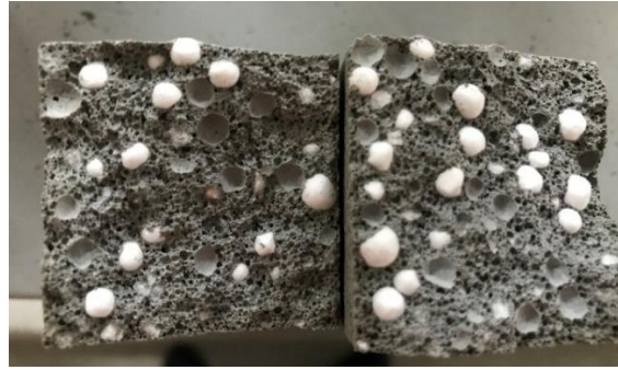
Figure 1. Sample of foam concrete after flexural strength test
