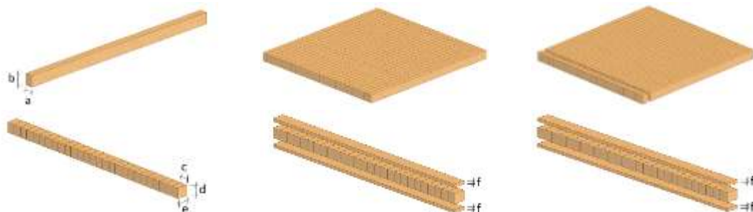
Figure 2. The process of preparing test samples (a: 14, 28 ve 42 mm; b: 22 mm e: 20 mm; d: 16 mm; c: 14, 28 ve 42 mm; f: 5 mm)
