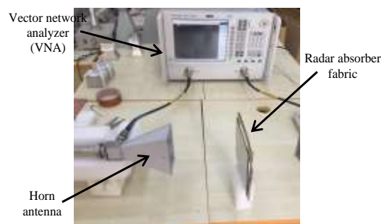
Figure 15. Frequency dependent reflection parameter measurements of planar radar absorber fabric
