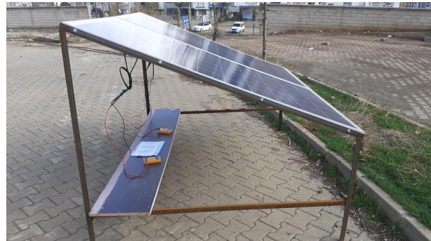
Figure 3. Measurement of short circuit current and open circuit voltage
