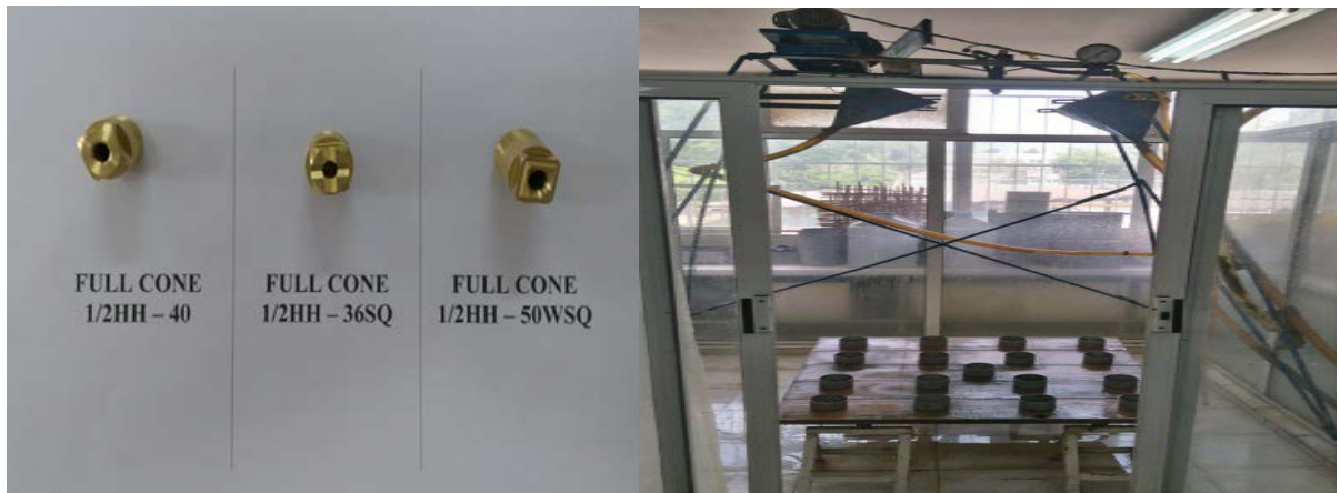
Figure 1. Full Jet type spraying nozzles, laboratory type rainfall simulator and cups used in experiment.
