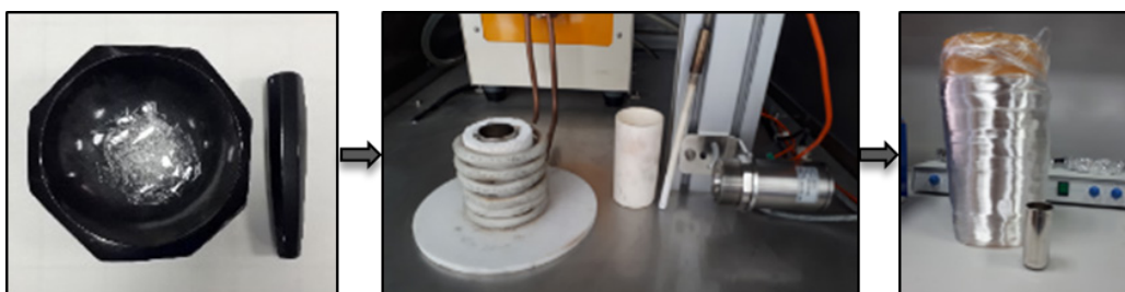
Figure 2. The production steps of the borosilicate glass fiber: breaking into small pieces, remelting, and drawing, respectively.
