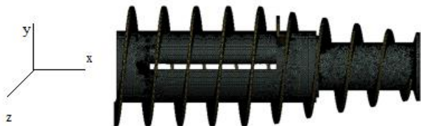
Figure 5. The Asymmetric Bladed Rotor Meshed Model
