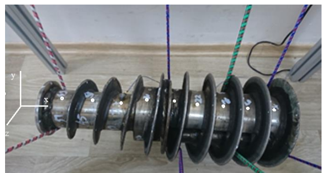
Figure 2. The Asymmetric Bladed Rotor with Free-Free Boundary Conditions
