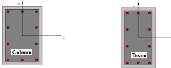
Figure 2. The cross-sections of columns and beams
