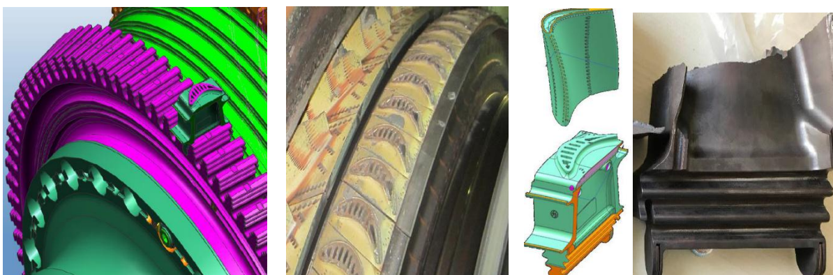
Figure 4. Broken blades on F-type unit
