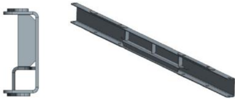
Fig. 8 Left, Bumper Cross Section. Right, Bumper
