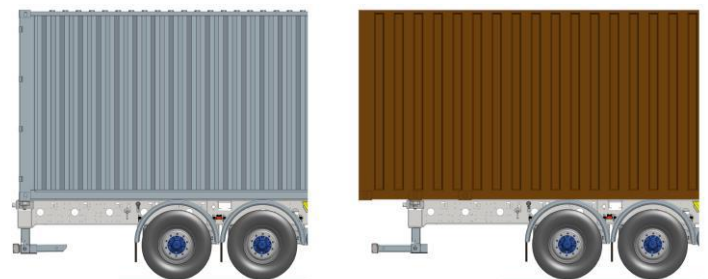
Fig. 4 Container Chassis Loaded with 40 ft. (left) and 45 ft. (right) Containers.
