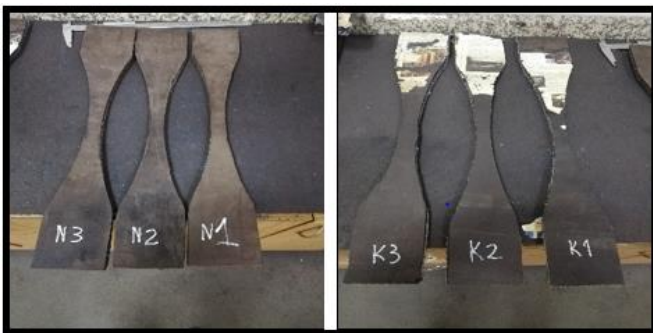
Figure 7. Bowtie-shaped specimens: Original unspliced (N coded) and vulcanized (K coded) belt specimens.
