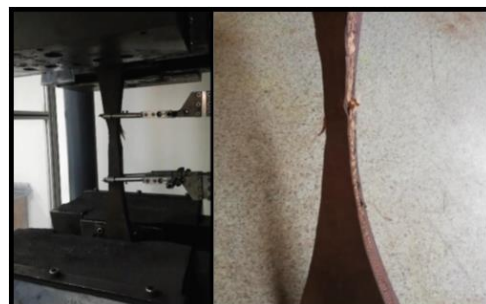
Figure 12. Tensile test image of the unspliced belt
