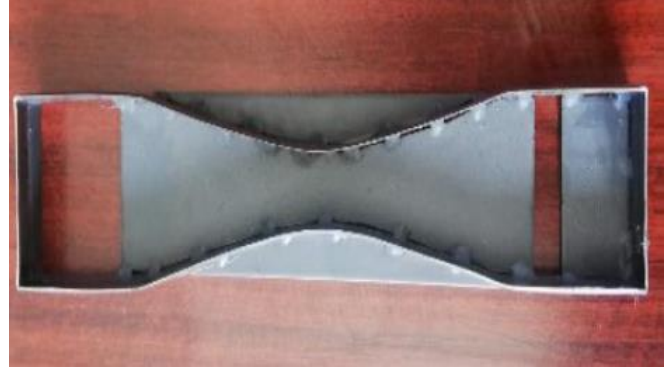
Figure 1. Image of bow tie specimen apparatus according to ISO 37 Standard [13]
