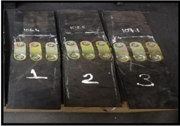
Figure 9. Image of belt specimens with mechanical splicing
