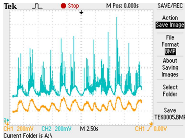
Figure 5. The rectified sEMG and envelope (top to bottom)
