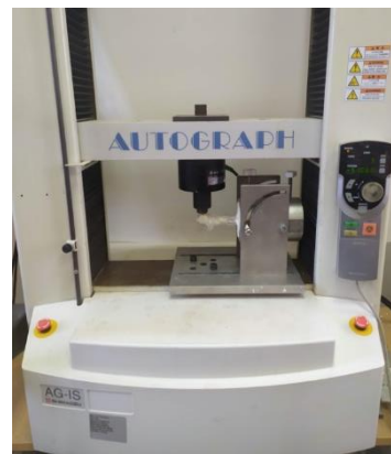
Figure 3. Biomechanical testing of a Sawbone® with Mayo 2A olecranon fracture fixation
