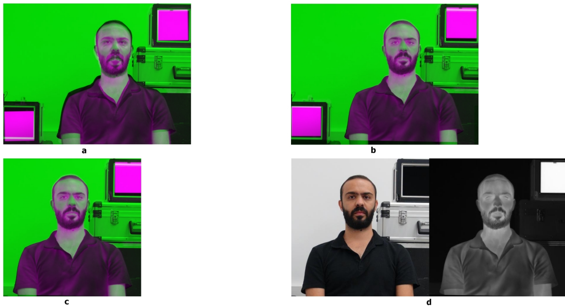
Figure 9. a) Acquired IR and visible images taken from cameras on top of each other using imshowpair method in matlab environment, b) superimposing images using pixel-by-pixel matching methods, c) display of mapped and cropped images for use in dataset with imshowpair method, d) representation of the visible and ir image pair to be used in the dataset
