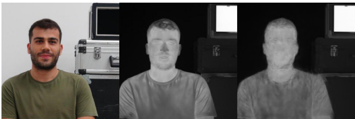
Figure 12. Best experiment result with never trained face image (left to right: visible real image, infrared image and fake infrared image)
