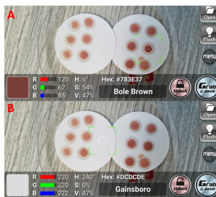
Figure 3. A smartphone app, 'ON Color Measure,' analysis process with the RGB model.
