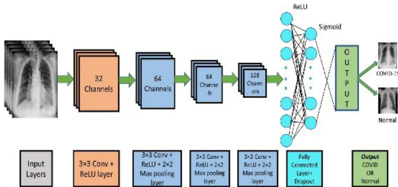
**Figure 2.** CNN architecture
