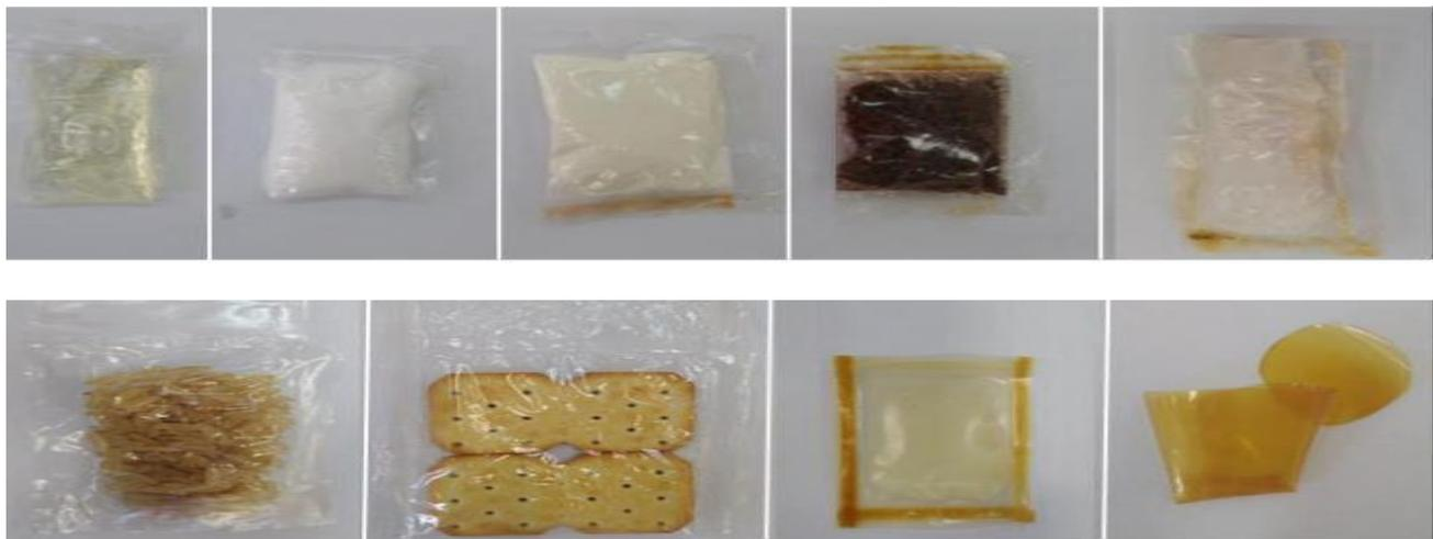
**Fig. 2** Different packages prepared by the bio-plastics/bio-films produced by the alginate.
