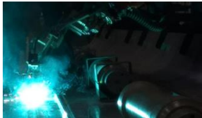
Figure 7. Tandem welding processes in TURASAS.
