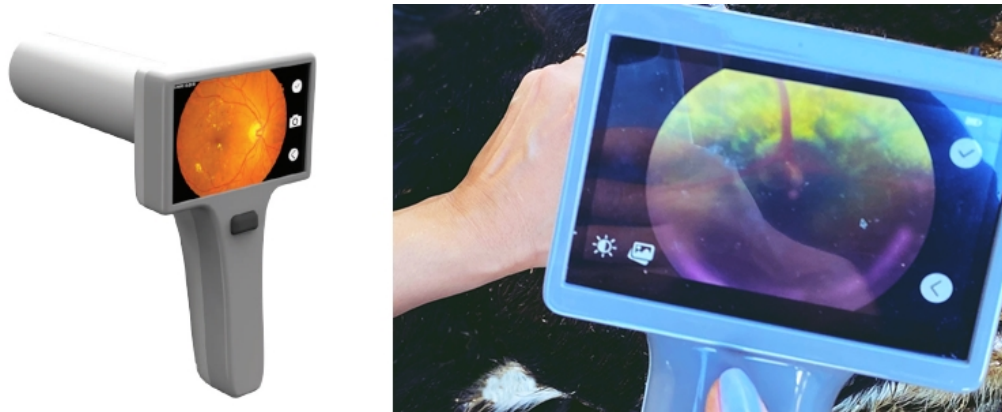
Figure 1. Fundoscopy with a non-mydriatic portable fundus camera.
