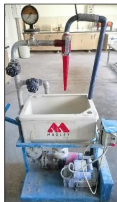
Figure 8. Mozley laboratory scale hydrocyclone and apex apparatus
