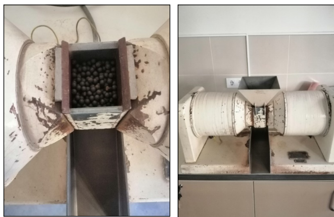
Figure 9. Carpco laboratory scale wet high intensity magnetic separator
