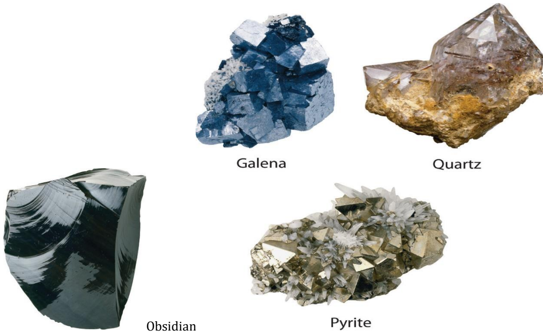
Figure 1. Galena( \text{PbS} ), Pyrite( \text{FeS}_2 ) and Quartz have crystal structure and obsidian is an amorphous material, (General Chemistry Notes)
