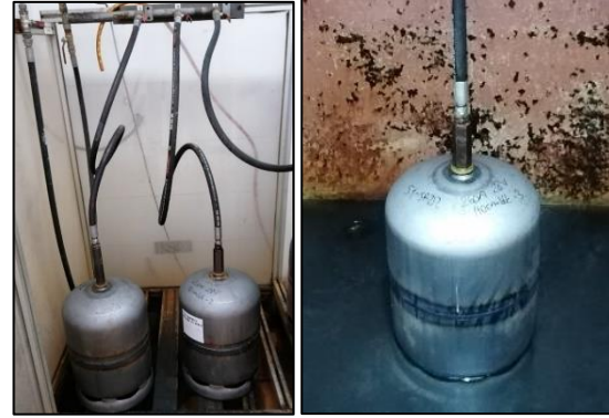
Figure 3. a) Bursting & volumetric expansion test set-up, b) Pressure fatigue test set-up
