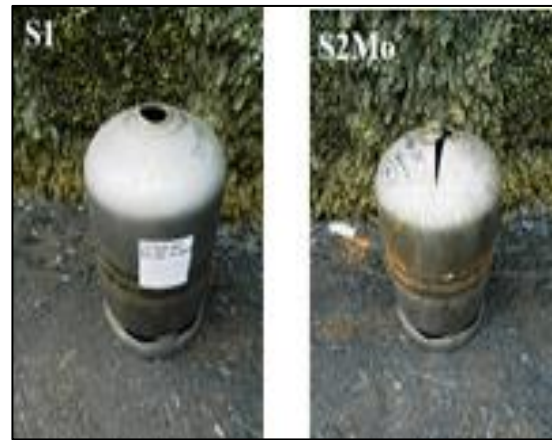
Figure 5. Cylinders subjected to bursting & volumetric expansion test
