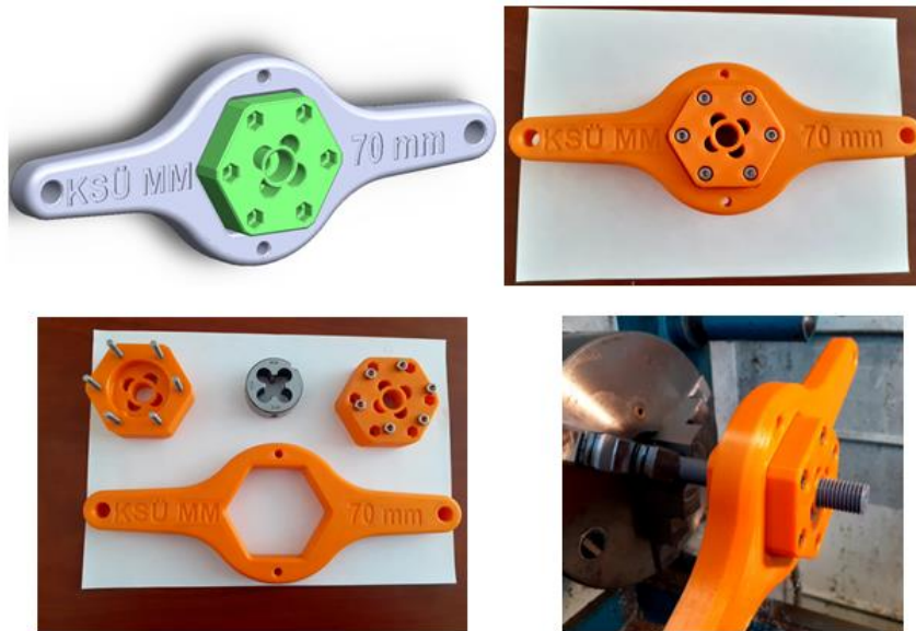
Figure 3. Design and produced novel threading tool
