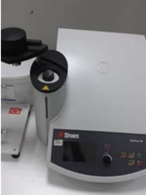
Şekil 9. Struers Citopress-10 bakalite alma makinesi (Figure 9. Struers Citopress-10 leveling machine)
