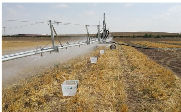
Figure 5. WCC lined up under the boom
