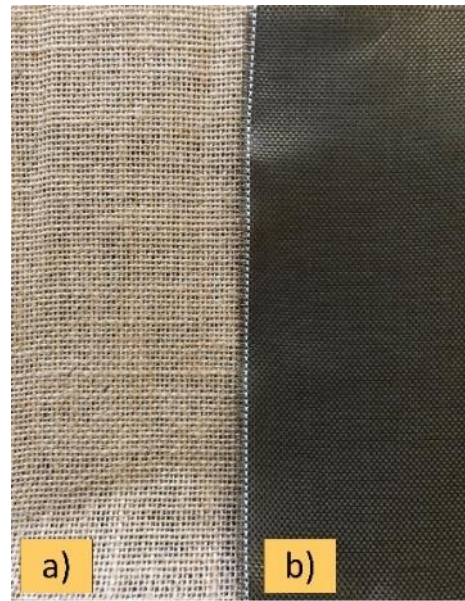
Figure 1. Fabric specimens: a) Jute fabric b) Basalt fabric
