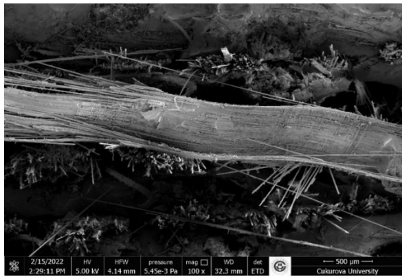
Figure 17. JBE composites at 90°C post cure temperature SEM micrograph
