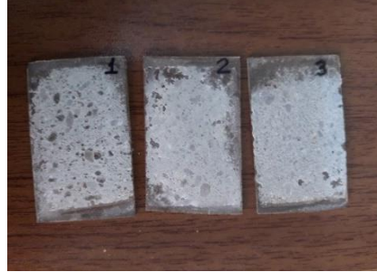
Figure 2. Thin sections extracted from specimens for petrographical analysis
