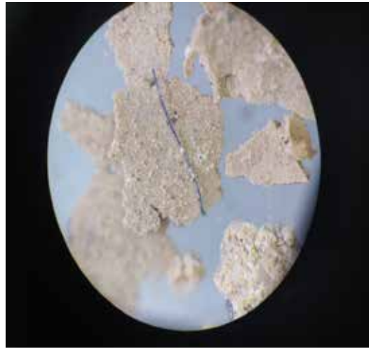
Figure 1. Microplastic appearance of soil with mineral part after H_2O_2 application
