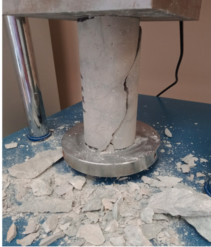
Figure 13. A rock sample failed under the UCS test
