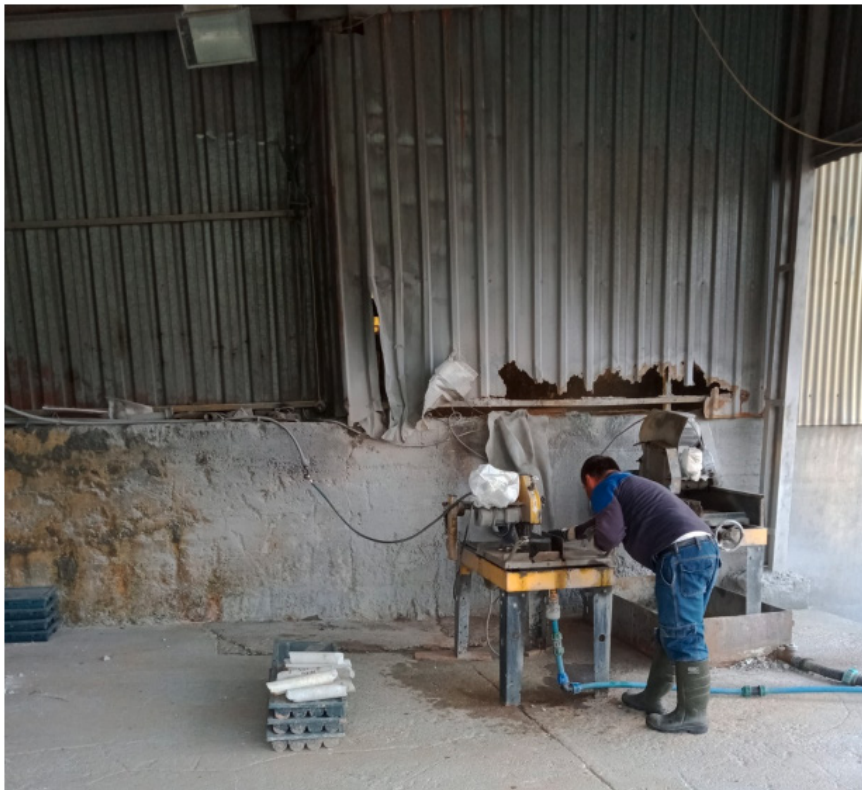
Figure 12. Rock core sample cutting by using the sawing machine
