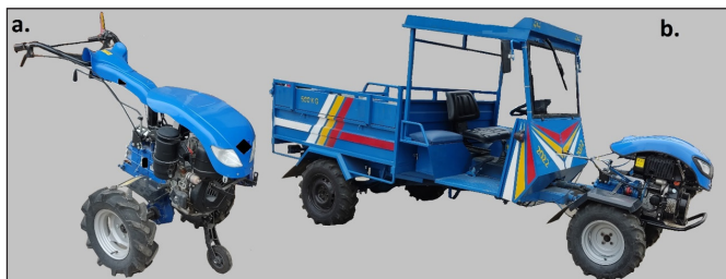
Figure 1. The design of the Pat-Pat vehicle (a) The two-wheeled Pat-Pat, which is designed as simple gardening digging-riding equipment. (b) A simple chassis, seats, and a 2-wheel trailer are added to the back to obtain a simple four-wheel drive Pat-Pat vehicle. (The vehicle in the photos belongs to the author's father and the author took these photographs himself. The author has the right to use the photographs.)
