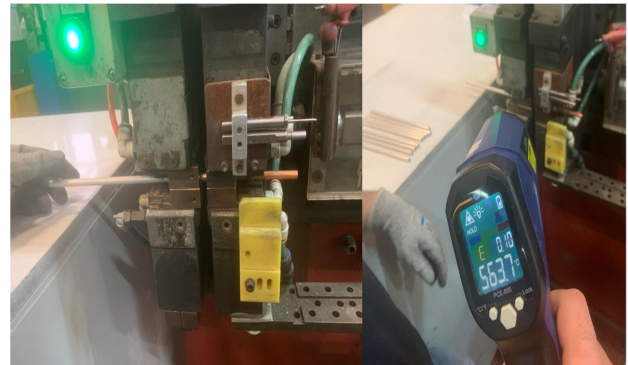
Figure 5. Combination of aluminum and copper tube and temperature measurement.
