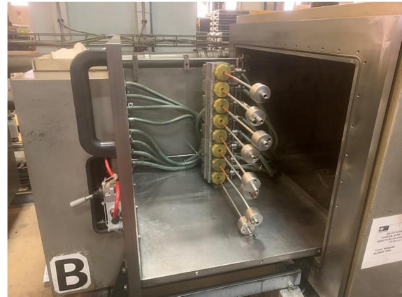
Figure 14. Connecting the samples to the leak tester.
