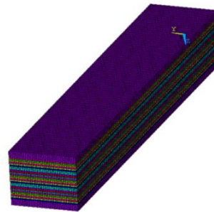
Fig. 2: The finite element model of an FGP sandwich beam
