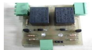
Fig. 11: Air Pump Motor Driver
