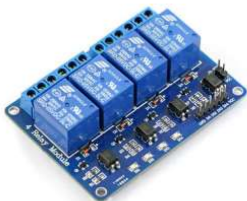
Figure 5. 5V Four-Channel relay module
