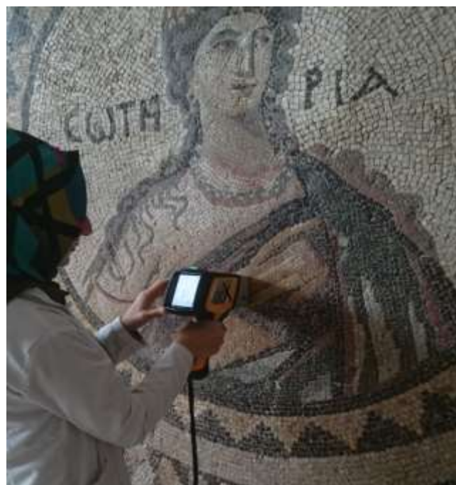
Figure 2. The process of analyzing samples with the P-EDXRF instrument.
