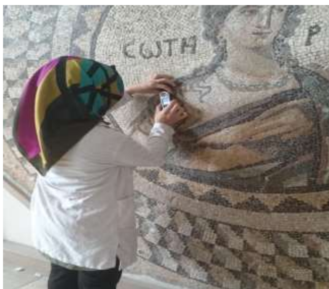
Figure 5. X- Color analysis with Rite CAPSURE device
