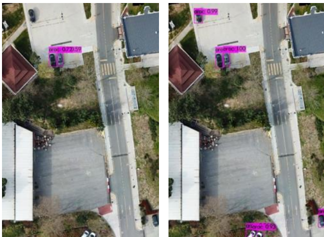
Figure 6. Evaluation result on test area 1 (YOLO-v3 on the left; YOLOv4-CSP on the right)
