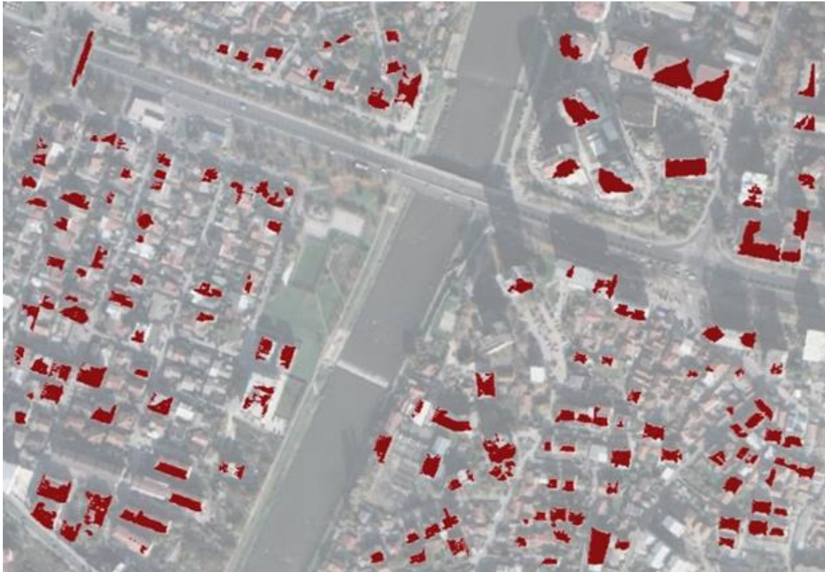
Figure 10. Identified red polygons that represent roof planes suitable for a solar PV system
