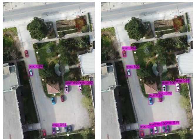
Figure 7. Evaluation result on test area 2 (YOLO-v3 on the left; YOLOv4-CSP on the right).
