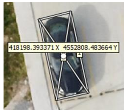
Figure 8. Obtaining the midpoints of the vehicles via Agisoft Metashape software
