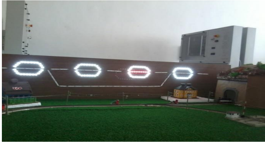
Figure 11. Monitoring of train location (red colour strip led) on CTC board
