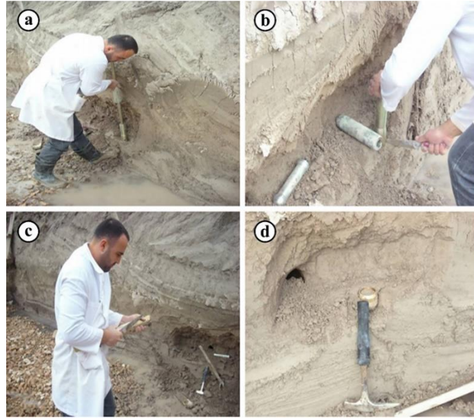
Figure 2. a) Tube sampling with sampling device, b) cleaning the outer side walls of the tube samples, c) waxing of the upper and lower parts of the tube samples, d) undisturbed soil sample image was taken into the consolidation ring.
