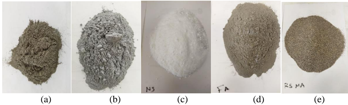
Figure 3. Mix materials a) Cement, b) SF, c)NS, d)FA and e)micro aggregate
