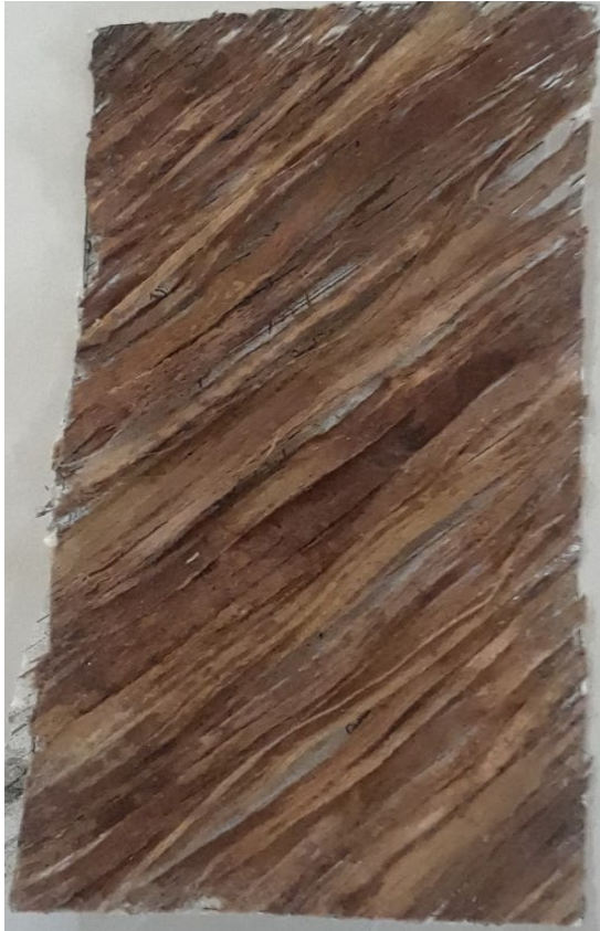
Figure 1: Fibre placed at 30° angular orientation
