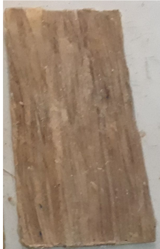
Figure 2: SSD fibre/PTE wood dust epoxy composite fibre placed at 0° angular orientation
