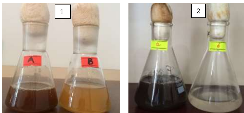
Figure 1. The color change of reaction mixture during the formation of silver nanoparticles by Candida macedoniensis BSU -MI44: a- experiment, b-control (1- 25°C, 2 - 30°C).
