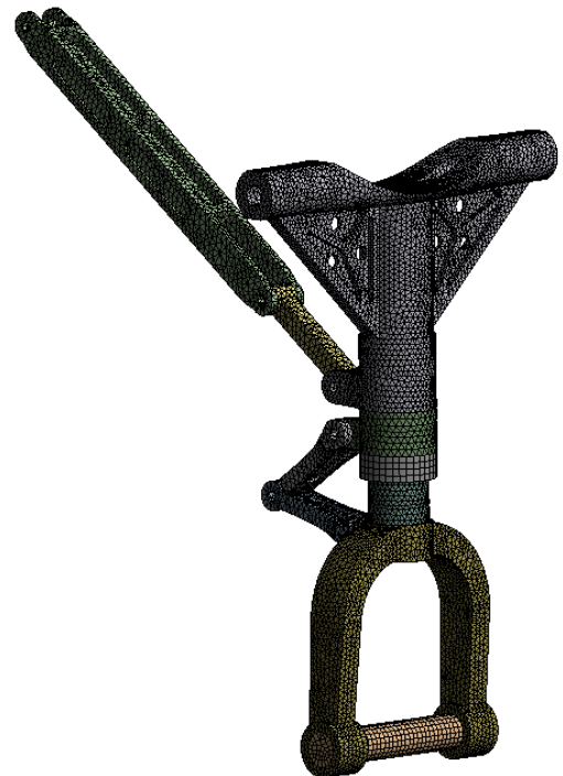
Figure 5 Mesh of FE Model
