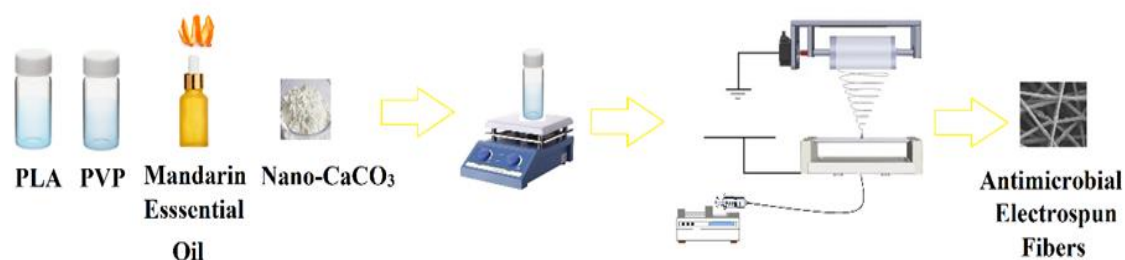
Figure 1. Schematic representation of the fabrication of bioactive composite electrospun webs
